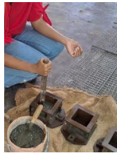
Fig. 2. Compacting each 50mm layer with a compact bar
