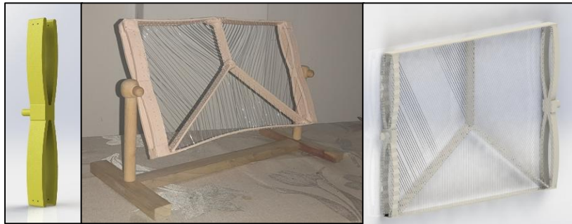
Fig. 6. Fabricated 1:3 model using the double wishbone members (left) and the rendered model (right)
