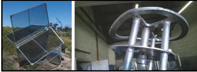
Fig. 4. Wind damage to the Whirly Mk II (left) and to the aluminium drive ring (right)
