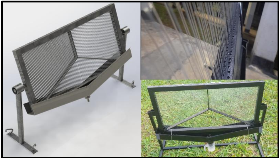
Fig. 5. Design and Fabricated small fog collector (600 mm 2 ) exhibiting the triple mesh and rotatable mesh frame
