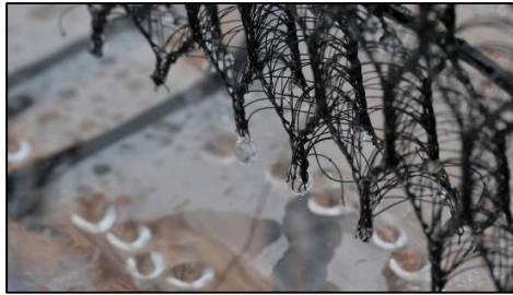
Fig. 1. 3D spacer mesh used in a commercial fog harvester (copyright: aqualonis )
