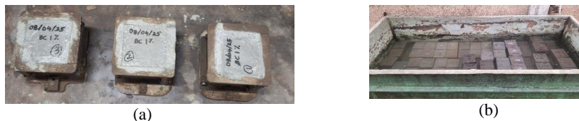
Fig. 3. (a) Dried RHB 1wt% integrated concrete blocks with mould; (b)Curing water bath.
