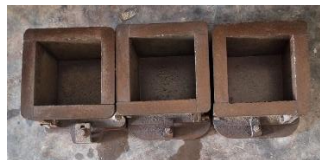
Fig. 1. Oil & grease applied (150×150×150mm) mould
