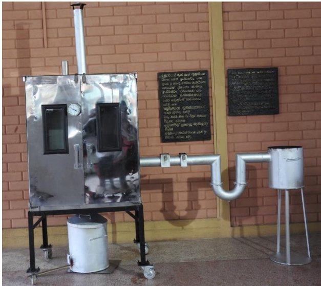
Smoked fish processing unit
